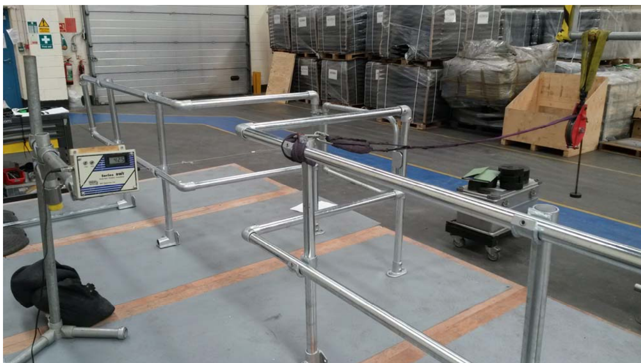
Plate 2 - Load Application and Deflection Measurements System
